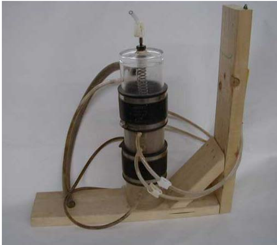
Figure 5-24. Rigid wall permeameter (Photograph courtesy of GeoComp Corporation).
