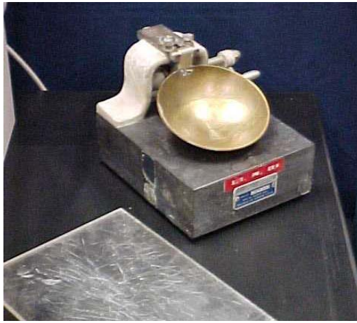
Figure 5-4. Some of the equipment used for Atterberg limits testing of soil.
